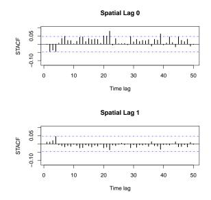
Figure 8: Space-time Autocorrelation Function (STACF) of the residuals from the fitted STARMA $(4_{1,0,0,0}, 0)$  model.
